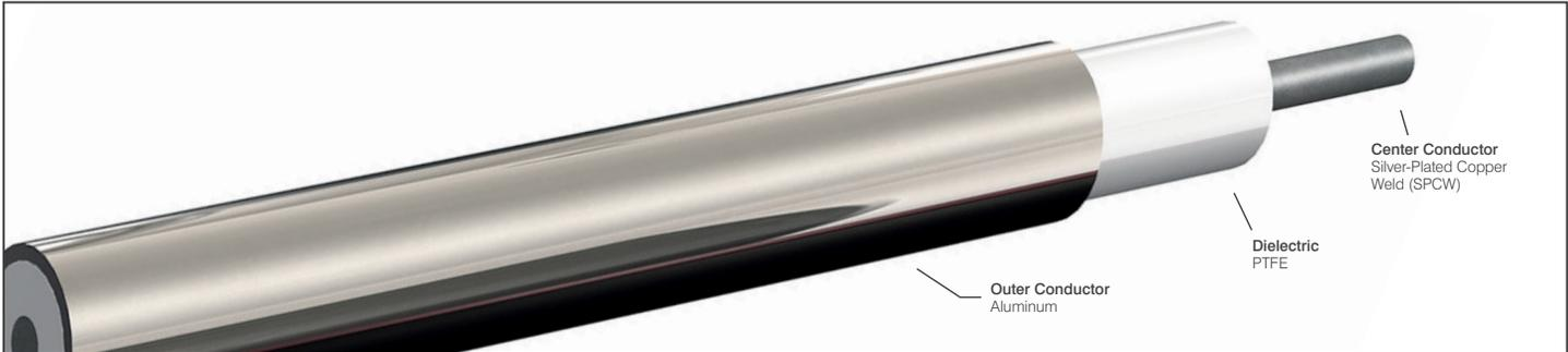
Our 50 Ω aluminum semi-rigid cables are ideal for hand forming or where weight savings is a premium.
