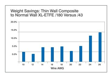
Composite Wire can save between 2% and 15% weight compared to XL-ETFE.
