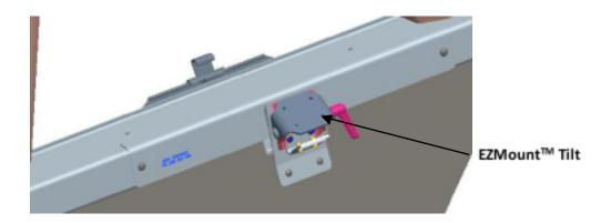
FIGURE 2 - CAPTAIN SIDE WINDOW MODIFIED WITH EZMOUNT™ TILT (FIRST OFFICER INSTALLATION IS MIRROR IMAGE)
