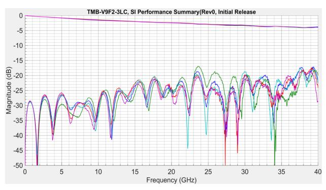
\* 10 connectors are shown, measured in pairs. (5 measurements) For further details regarding testing setup, configurations please see the rest of the report.
