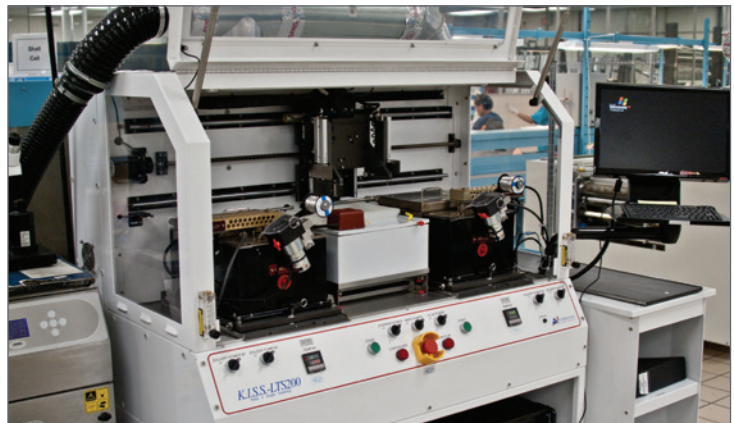
Automated solder dip equipment
