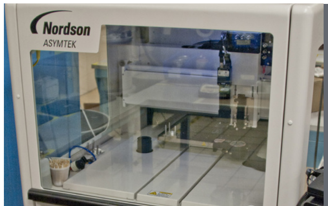
Automated potting controls process and quality
