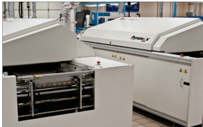
Zoned ovens ensure control over solder reflow
