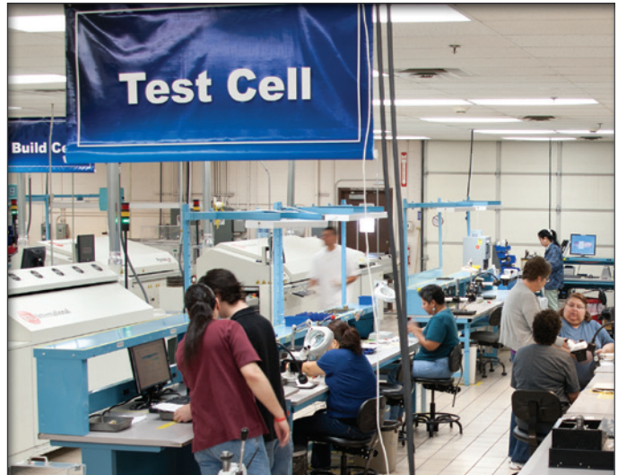
Burn-in, thermal shock and thermal cycle testing available in-house
