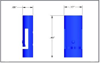
Patented Contact Retention Mechanism
