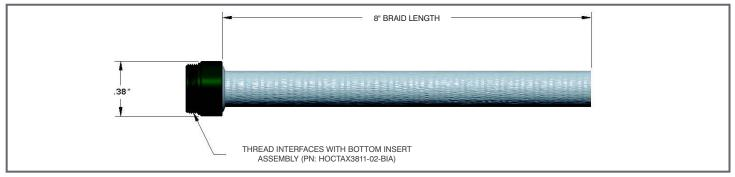
• Aluminum parts are cadmium plated per AMS-QQ-P-146. Braid Material is P/N AA59569R36T0250
