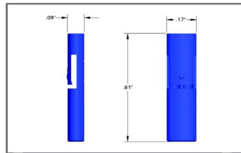
Patented Contact Retention Mechanism
