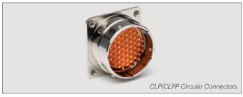
Our CLP/CLPP Circular Connectors are ideal for blind-mating in IFE (In-Flight Entertainment) systems and aircraft galley applications where intermateability with MIL-C-26500 is preferred. These connectors will readily mate with MIL-C-26500 bayonet-type plug MS24266R series connectors and can be PC board-mounted.
