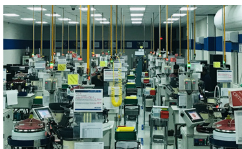
Automated Plating Lines (Full Plating & Selective Plating)
