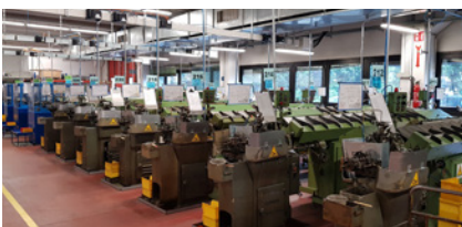
Blank Manufacturing using Cold Heading and Screw Machine
